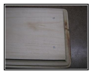
Drill 2 1/16" pilot holes: For the 2 #4 screws that hold down both the lever AND the FUNKeyer printed circuit board.
